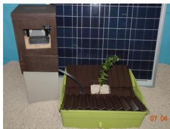
Figure 6- Irrigation system for plants and trees that take the water from humidity of the air.
