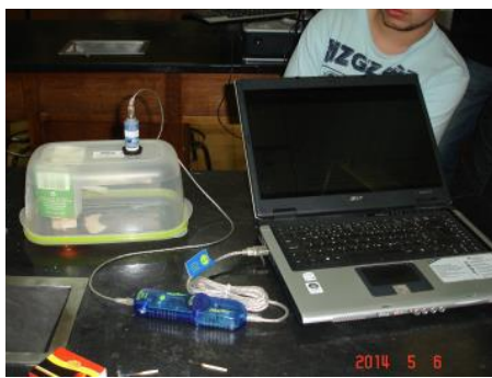
Figure 4- Device for measuring the concentration of oxygen.
