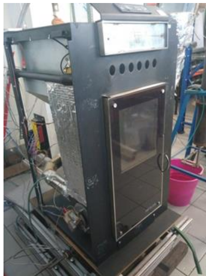
Figure 1. Boiler used in the experimental work.
